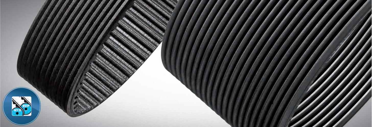
The **optibelt OMEGA RB** differential timing belt features a RB belt ground into the back-side. This creates a unified belt that will not separate. The belts are used primarily in mills where the back pulley has a reversible direction. The RB backside will allow for slippage if the machine becomes blocked or locks-up.
