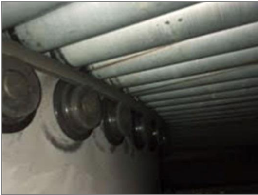
Conveyor v-belt drive configuration. In this application the top of the v-belt provides the force for the rollers.
