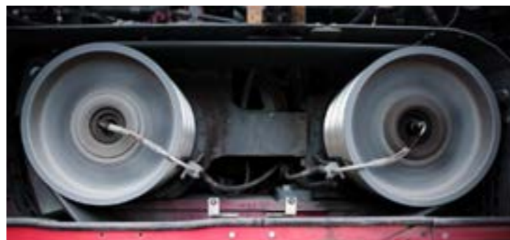
OPTIBELT 5V KB Kraftbands drive both motors forward
