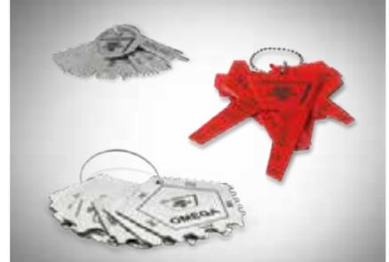
Valuable help for the measurement of belt and pulley profiles
