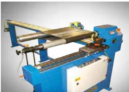
The **optibelt CUT II** belt slitter was specifically developed for modern storage for the technical trade.
