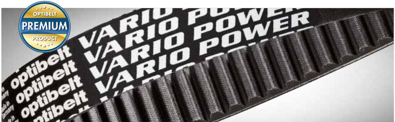
The base compound consists of a poly-chloroprene rubber compound with fibres inlaid transversely to the running direction. The high-quality and extremely low-stretch polyester or aramid tension cord is embedded in a cushion compound. It is reinforced with a fabric outer surface, and the transverse fibres incorporated provide transverse rigidity without sacrificing flexibility.
