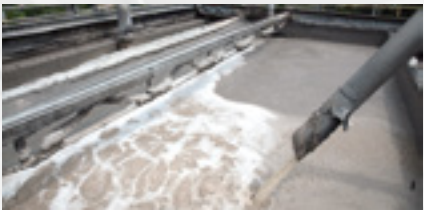
1. PULPER (PULP PRODUCTION) Pulp and waste paper are mixed with water and broken down into separate fibres.
