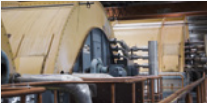
4. PRESS Water is then carefully removed from the wet paper web.
