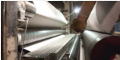
5. SMOOTHING Steel rollers smooth the paper ready for further processing.
