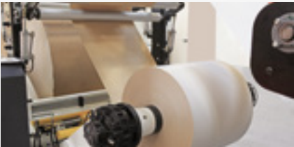
8. REEL STAND A powerful drive system ensures a quick and flexible output.
