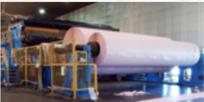
7. WINDING ONTO ROLLS The paper web is wound onto a tambour in various widths.
