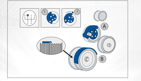
Mounting tool for OPTIBELT elastic ribbed belts
